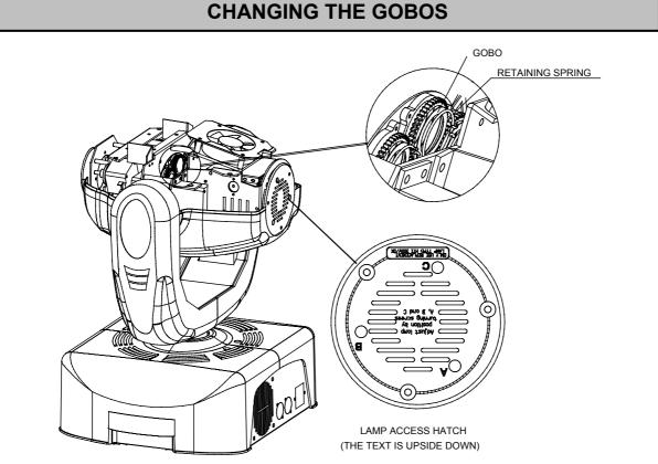
Carefully lift off the plastic cover by undoing the 4 M4 screws. (**NOTE:** The projector has two covers with the same shape. The cover removed must be right one, so you can change the gobos easily. How to remove the correct cover, the easy way is to position the projector with the text of the lamp access hatch upside down as shown above, and then remove the upper cover.)
