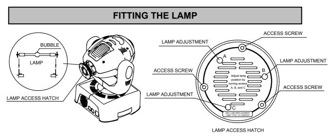
Loosen the 3 access screws at the rear of the projector and pull the lamp access hatch straight out from the rear of the projector. Insert an HTI 300W/DX lamp in the lamp holder. Close the lamp access hatch, then tighten the 3 access screws.
