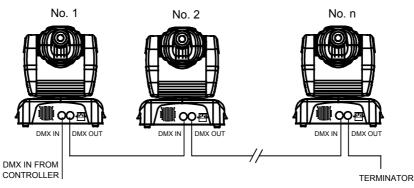
PILOT 300 uses 3-pin XLR plug / socket. If your controller uses 5-pin XLR plug / socket, you should use a conversion cable from 5-pin to 3-pin as shown bellow.
